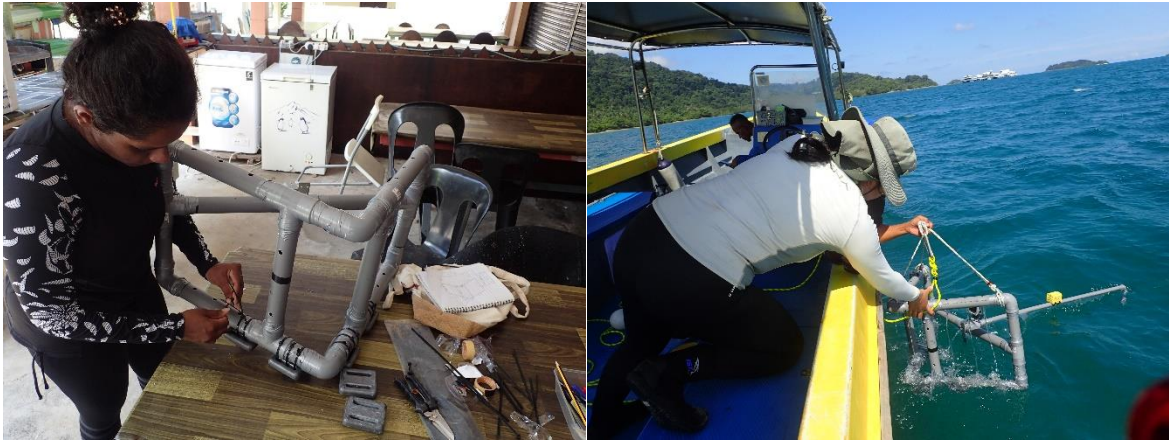
(Left) In the subtidal sites, a PVC setup was built as shown by MarAlliance . (Right) These were then deployed off the boat using ropes
