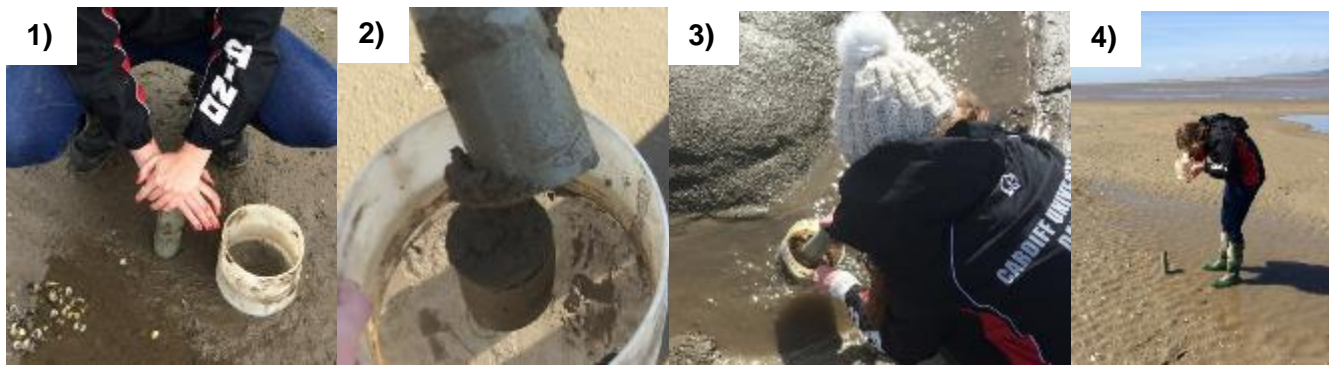
Figure 8 The process of coring; 1) Cores taken randomly (alongside random point sampling) with a standard PVC seed corer (50mm diameter x 250mm long) and cap (Mckenzie et al. 2003), pushed approximately 10cm deep into the substratum; 2) Sediment placed in stainless steel sieve (1-2mm mesh); 3) Sieved sediment using a little water and 4) Analysis of core content, where the number of whole seeds and half seeds retained was recorded. Seeds were then returned to the sediment to reduce core-induced disturbance. Image source: authors own, 2016.
